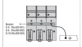
Multiple products installation, busbar E-3, E-5 or E-10 can be used to combine all the earth terminals to earth.
